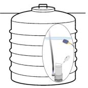
Delay the level at which a submersible pump fitted with a float begins to operate
